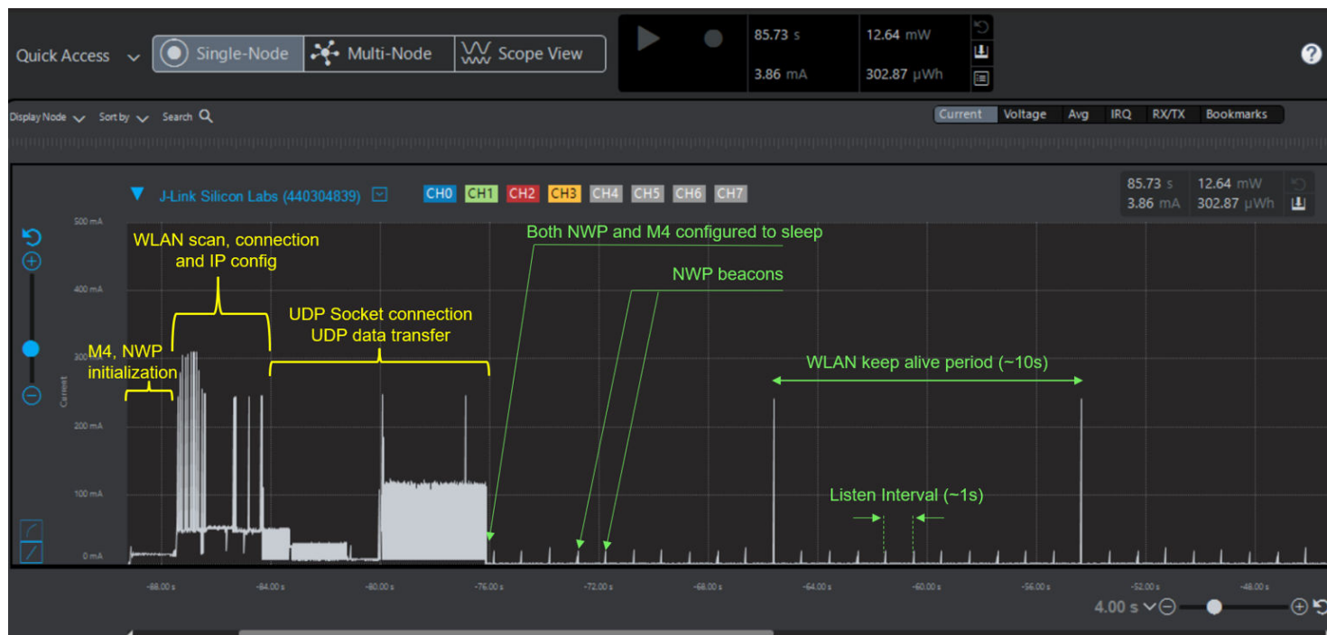
Figure 8.2. Powersave Standby Associated Example Current Consumption Graph
